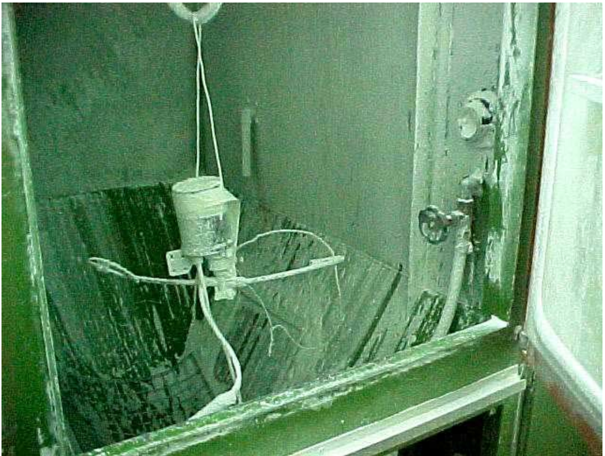
Fig. 1 Dust test set-up (subject unit in the dust chamber with a pipe for connection to vacuum pump)
