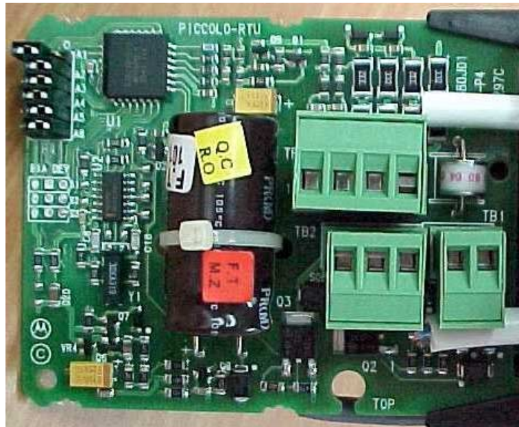
Fig. 3 Internal view of Sample 2 after dust test (no traces of dust observed)
